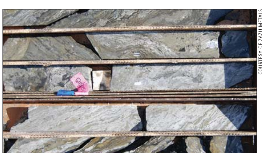
The photo shows core from hole 159 drilled in 2008 at the Lik property. The 26 meter intersection the core came from averaged 8.73 percent zinc and 2.75 percent lead.
